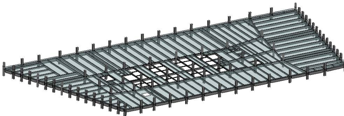
Figure 12–8. Typical tenant floor structural framing and slab model (Floor 8 to 20, 24 to 45)
